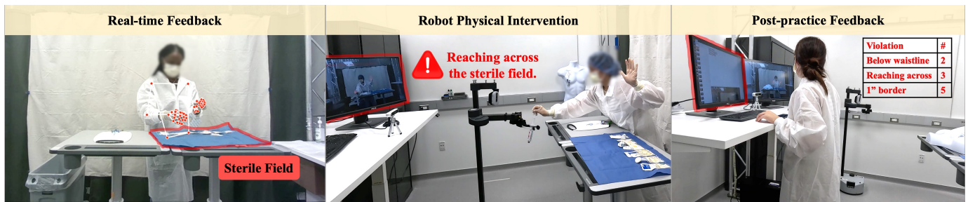
Figure 2. Nurses practicing dressing change procedures with ASTRID in a nurse training environment. ASTRID offers (left) real-time guidance, (middle) physical interventions, and (right) post-practice feedback to help nurses master “principles of sterile technique” for preventing healthcare-associated infections.
