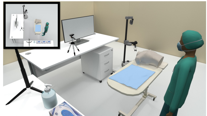
Figure 5. Artificial rendering of the training environment shown in Fig. 2, highlighting its key elements: nurse, simulated patient, medical supplies, and ASTRID (composed of the robot, depth camera, and computer screen).
